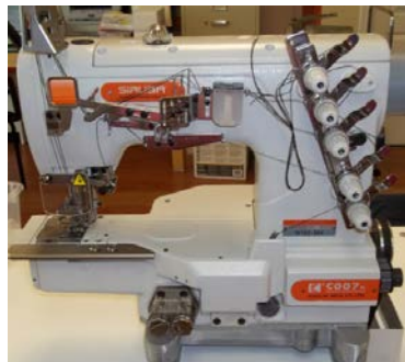
Pre-Threaded, 3 needle Cover Stitch Machine
